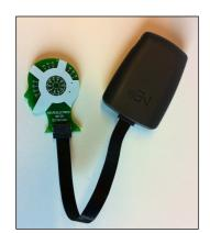
NE's test-board provides an electrical interface for simulation of EEG impedances and signals. Shown here attached to a
