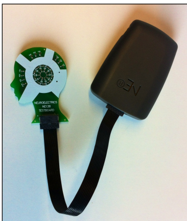
NEs test-board. Provides an electrical simulation of EEG impedances and signals.
